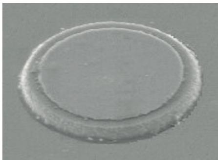
**Fig. 1 | The first GaN microLED.** Scanning electron microscopy image of one of the first microLEDs, which were based on indium gallium nitride/gallium nitride (InGaN/GaN) quantum wells. The device has a pixel size of 12  $\mu\text{m}$  and p-type nickel/gold (Ni/Au) contact diameter of 10  $\mu\text{m}$ . Figure adapted with permission from *Appl. Phys. Lett.* **76**, 631 (2000), AIP Publishing.
